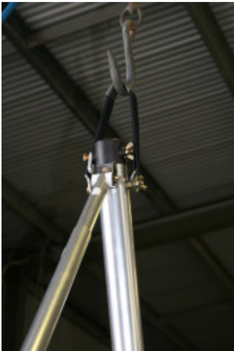
Figure 7 Tension the lifting apparatus while separating the trike base from the crate floor
