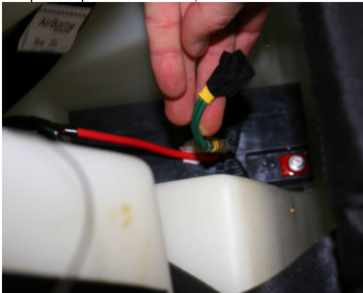
Figure 19 Connect the positive terminal of the battery
