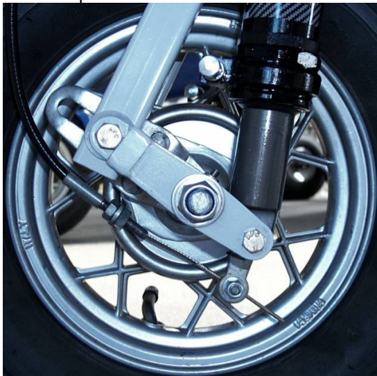
Figure 16 Front drum brake with torque arm
