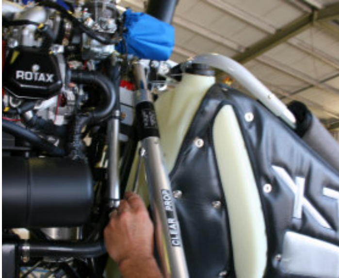
Figure 13 Install the compression strut
