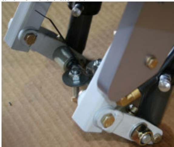
Figure 8 Unbolt trike from crate floor
