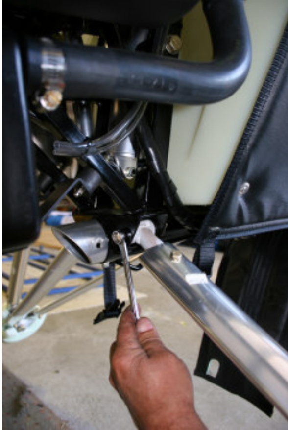
Figure 11 Connect lower wishbone struts, all bolts are inserted from the rear, with nuts to the front
